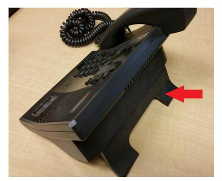
The coiled cable should plug into the bottom of the handset with the other end going to the jack on the phone located to the immediate left of the handset. The jack is labeled with the symbol:
